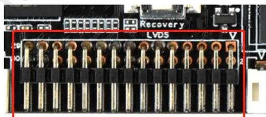
General LVDS interface definition, support single/dual, 6/8/10 bit 1080P LVDS screen. The screen voltage can be selected through the bridge-wire cap, and can choose to support 3.3V/5V/12V screen power supply.
